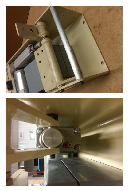
To adjust the retraction and extension you can turn the red and white screws on the end of the actuator. The Red screw adjusts the down position of the pushing arm. Turn the screw clockwise to make it arm retract further. The White screw adjusts the up position of the pushing arm, turn the screw counterclockwise to make the arm push further past 90 degrees. There are about +/- 10 turns of adjustment for each screw.
